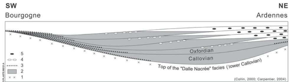
Fig. 4. – Thickness changes in the Callovian-Oxfordian clay formation from the Ardennes to the Burgundy swell, from Carpentier's [2004] well log correlations.
