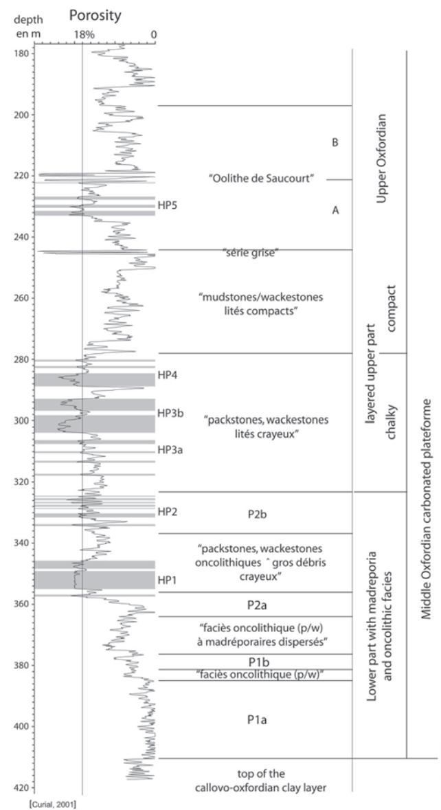
Fig. 8. – Vertical changes in the secondary porosity affecting Oxfordian platform carbonates in the ES 204 well.
