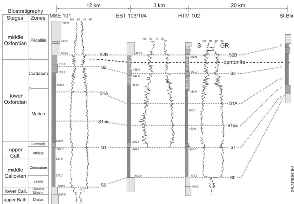
Fig. 2. – Stratigraphic position of the main key surfaces used for detailed correlations in the Callovian-Oxfordian clay formation at the scale of the Meuse/Haute-Marne area.
