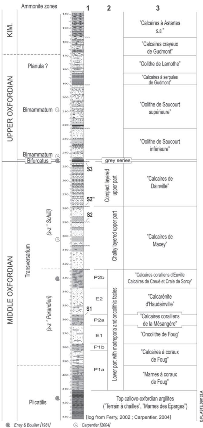
Fig. 5. – Detailed stratigraphy of middle to upper Oxfordian platform carbonates on the Andra site (well EST204).
