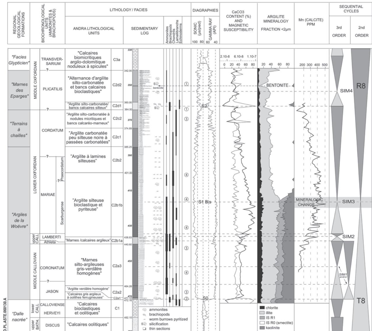
Fig. 3. – Sedimentology, mineralogy, geochemistry and sequence stratigraphic interpretation of the Callovian-Oxfordian clay formation in the Meuse/Haute-Marne area.
