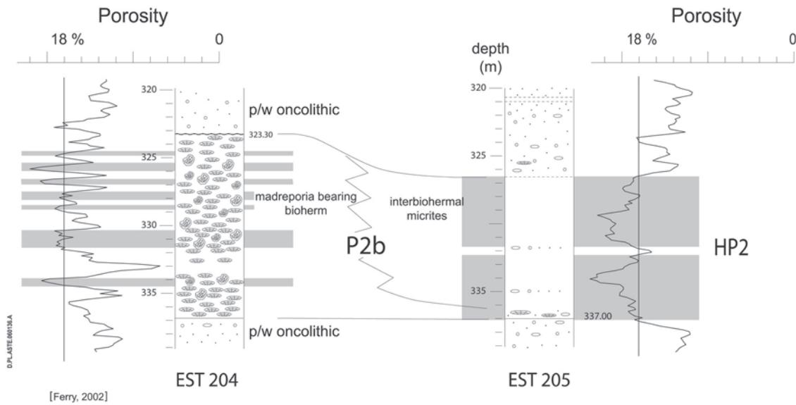
Fig. 9. – Porosity changes as a function of depositional facies between the closely spaced wells EST204 and EST205 on the Andra site of Bure. DIAGEVAL® porosity calculated from well log values [Andra, 2001]. Porous horizons HP as defined from neutron porosity values above 18%.
