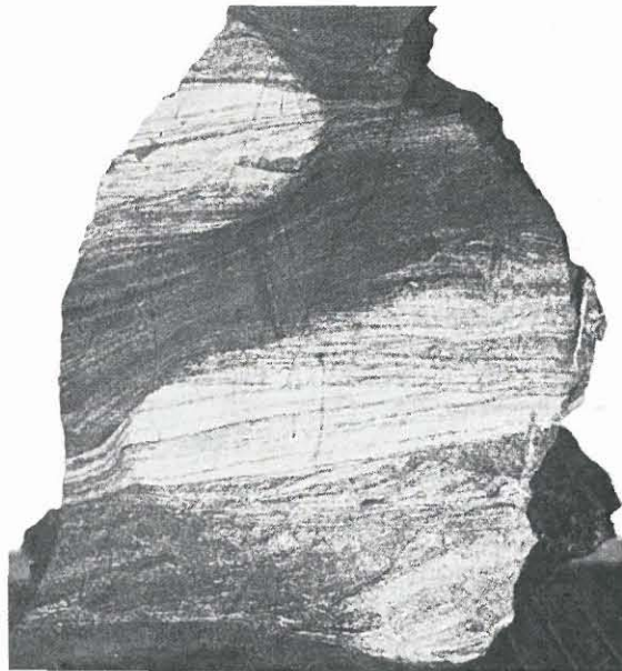
Fig. A-3. Calcite concretions. There is a continuity of the laminae between the concretion and the inter-concretionary ore. The inflection of laminae along contact with the two margins indicates a settling of the inter-concretionary ore material and increase in volume of the concretions during the process of \text{CaCO}_3 displacement; \times 0.25 .
