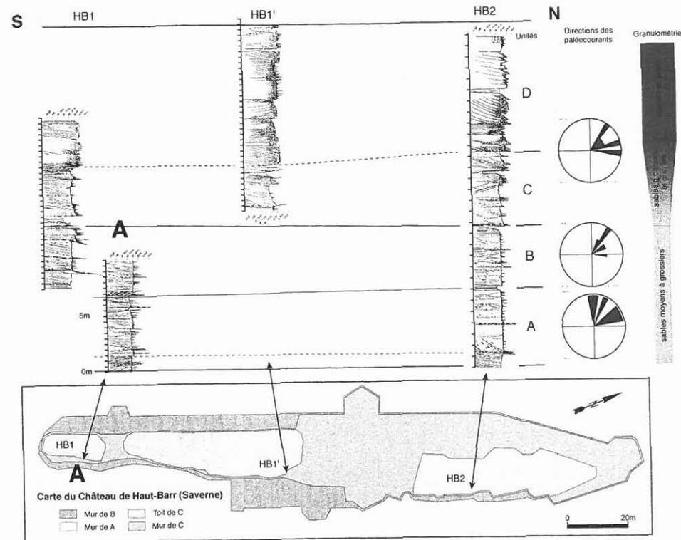
**Figure IV.3:** Sedimentological log of 'Grès vosgien' and 'Conglomerat principal' of the Haut Barr outcrop (after Guillocheau *et al.*, 2002)
