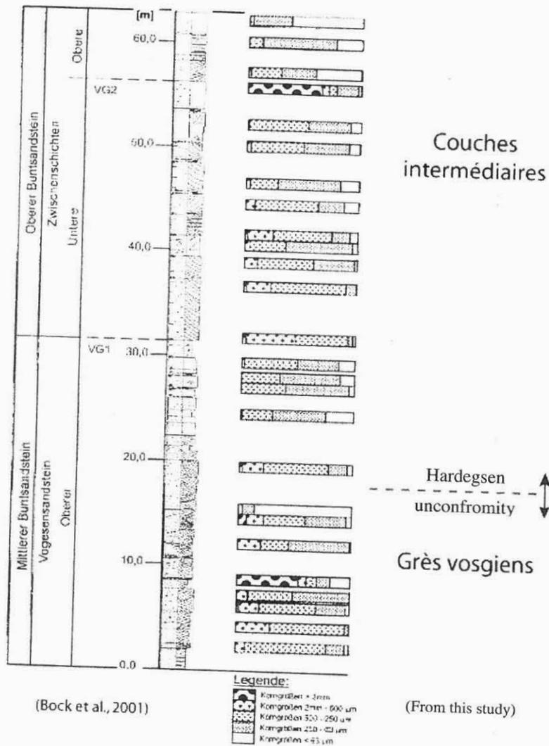
Figure IV.33: Sedimentary log of Bitche (Stop 3.1) by Bock et al. (2001) which differs from our observations. VG1 and VG2 are paleosol key-beds defined by Müller (1954)
